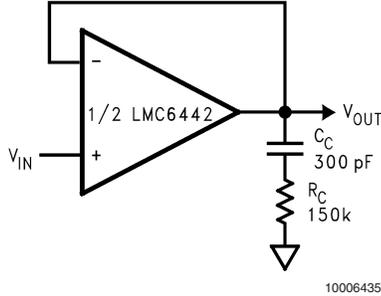
**FIGURE 1.  $A_V = +1$  Operation by adding  $C_C$  and  $R_C$**
