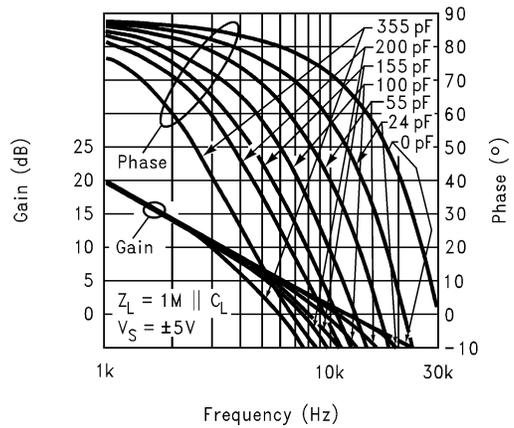
**Open Loop Gain/Phase vs. Frequency For Various C\_L (Z\_L = 100 KΩ || C\_L)**
