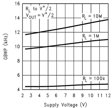
**Typical Performance Characteristics**  $V_S = 5V$ , Single Supply,  $T_A = 25^\circ C$  unless otherwise specified (Continued)
