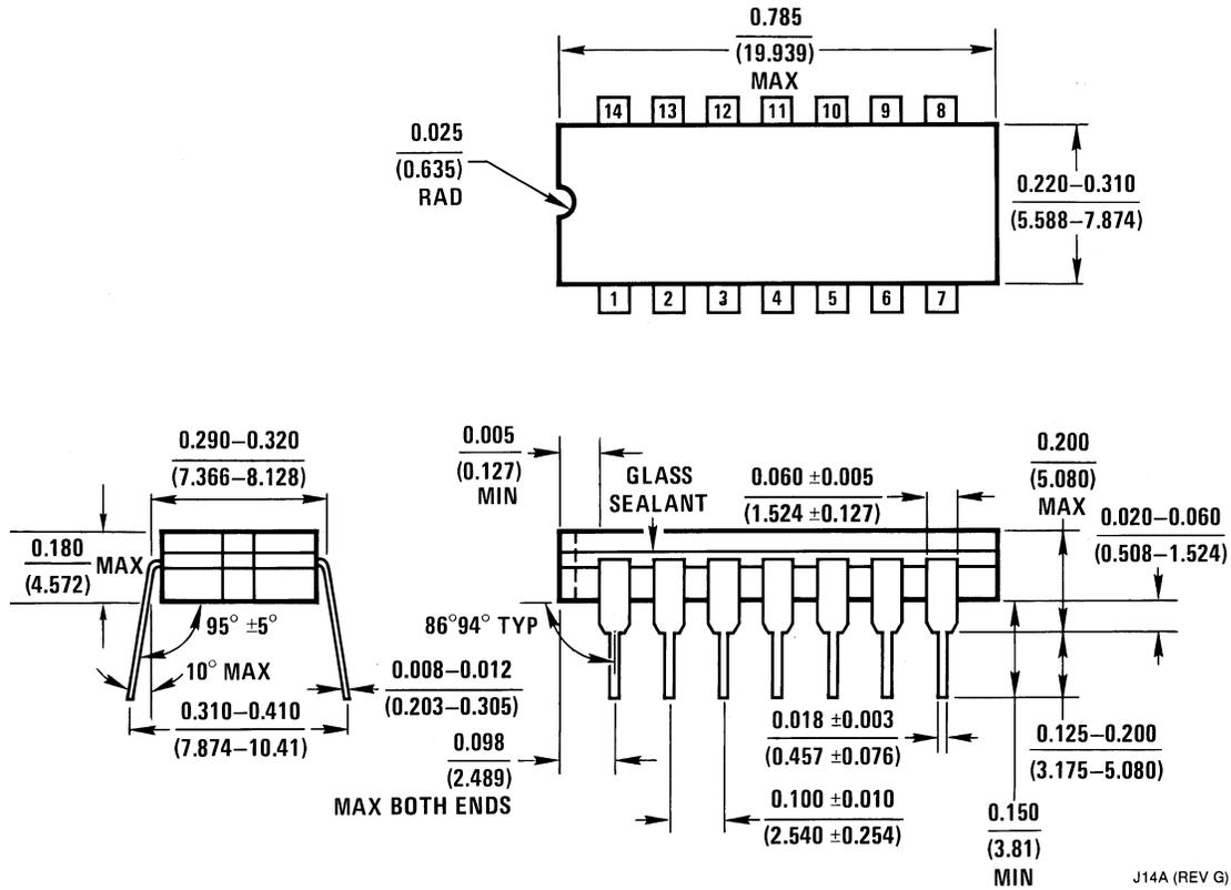
14-Pin Ceramic Dual-In-Line Package
