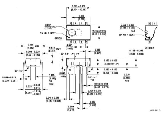
Molded Dual-In-Line Package (N) Order Number LMC568CN **NS Package Number N08E**
