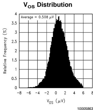
LMC2001 High Precision, 6MHz Rail-To-Rail Output Operational Amplifier
