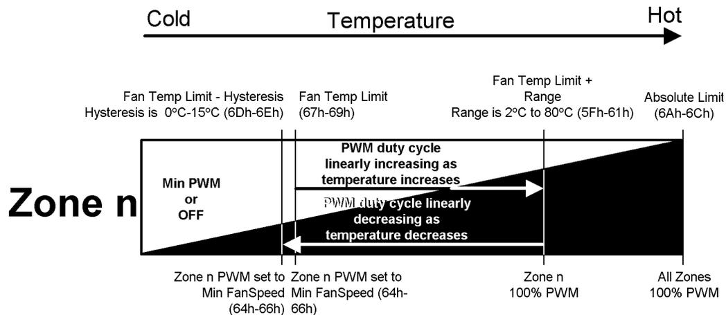
**FIGURE 1. Fan Activity above Fan Temp Limit**
