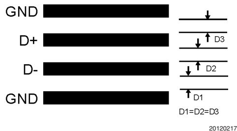
FIGURE 4. Ideal Diode Trace Layout
