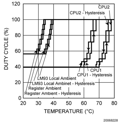
**FIGURE 1. Example of the LM93 Fan Control Transfer Function. Download an excel spread sheet from [www.national.com/appinfo/tempsensors](http://www.national.com/appinfo/tempsensors) that allows you to enter the fan control register values and then automatically generate a similar curve.**
