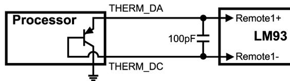
**Note:** 100 pF cap is optional and should be placed close to the LM93, if used. The maximum capacitance between these pins is 300 pF.
