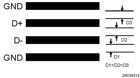
FIGURE 6. Recommended Diode Trace Layout
