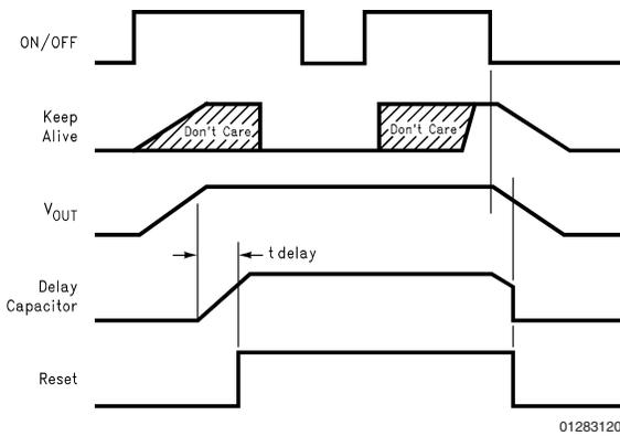
**Safety Latch OFF of  $V_{OUT}$  when in Keep-Alive Mode
