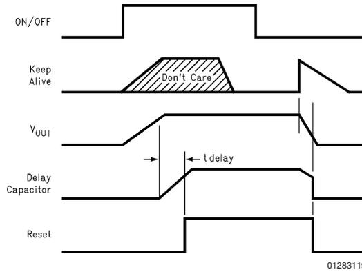
**Switch ON with ON/OFF input; Keep output
