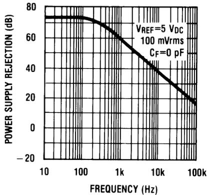
V<sub>CC</sub> Power Supply Rejection
