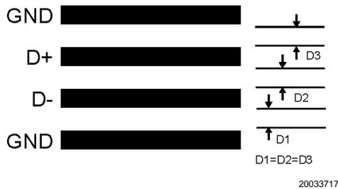
**FIGURE 15. Ideal Diode Trace Layout**
