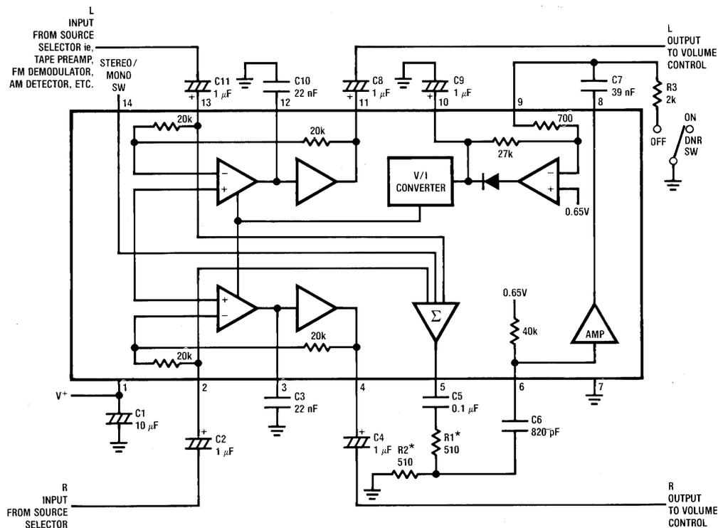
FIGURE 1. Component Hook-up for Stereo DNR System
