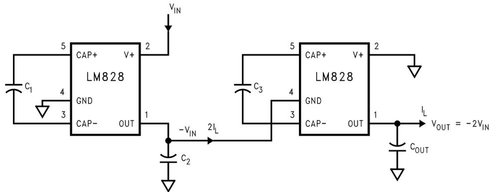
FIGURE 4. Increasing Output Voltage by Cascading Devices
