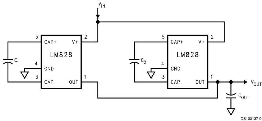
FIGURE 3. Lowering Output Resistance by Paralleling Devices
