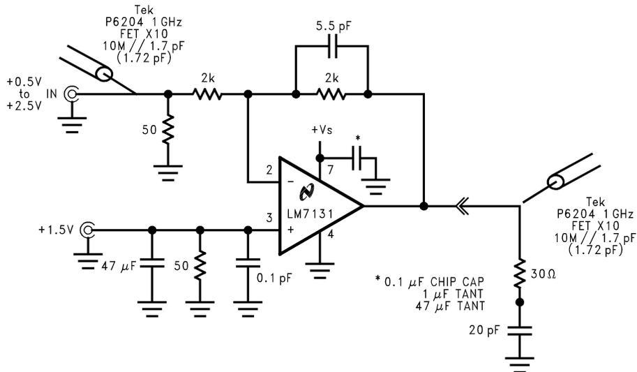
Numbers in parentheses are measured fixture capacitances w/o DUT and load.
