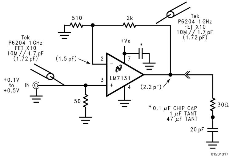
Numbers in parentheses are measured fixture capacitances w/o DUT and load.
