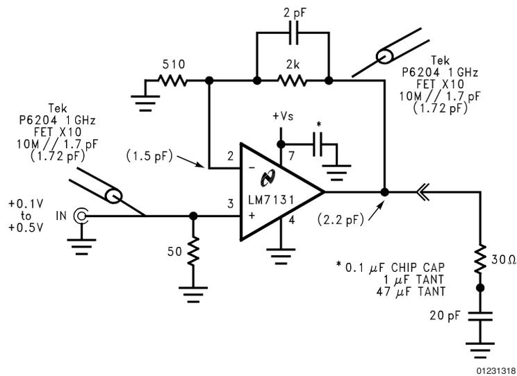
Numbers in parentheses are measured fixture capacitances w/o DUT and load.
