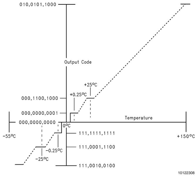
FIGURE 5. Temperature-to-Digital Transfer Function (Non-linear scale for clarity)
