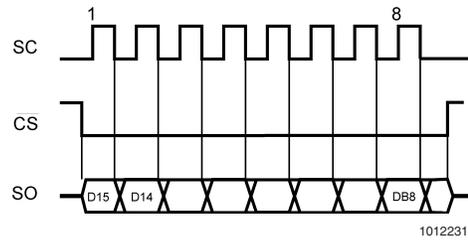
a) Reading Continuous Conversion - Single Eight-Bit Frame
