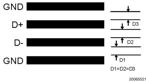
**FIGURE 11. Ideal Diode Trace Layout**
