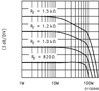
**BANDWIDTH vs  $R_f$  &  $R_S$**
