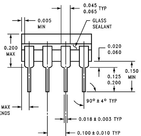
**8-Pin Ceramic Dual-In-Line Package**
