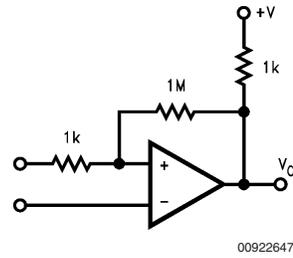
FIGURE 18. Comparator with Hysteresis ( $\Delta V_H = +V(1k/1M)$ )
