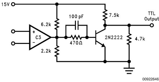
FIGURE 17. Wide-Input Range Comparator with TTL Output
