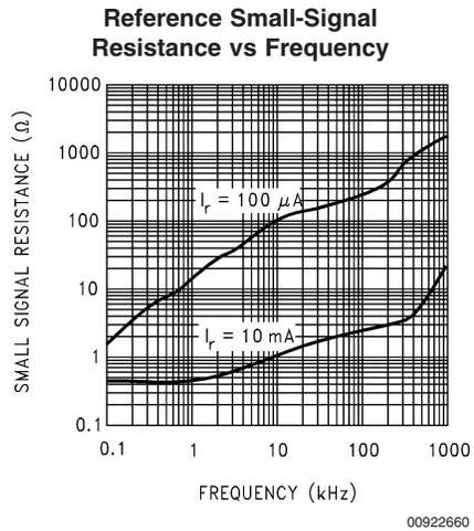
**Typical Performance Characteristics (Reference)**  $T_J = 25^\circ\text{C}$ , FEEDBACK pin shorted to  $V^- = 0\text{V}$ , unless otherwise noted (Continued)
