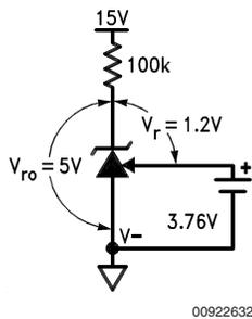
**FIGURE 4. Thevenin Equivalent of Reference with 5V Output**
