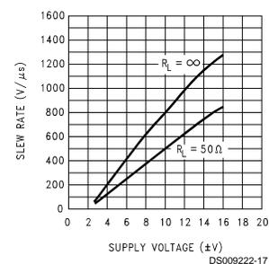
**Typical Performance Characteristics**  $T_A = 25^\circ\text{C}$ ,  $V_S = \pm 15\text{V}$  unless otherwise specified (Continued)
