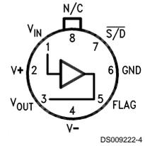
**Note:** Pin 4 connected to case
