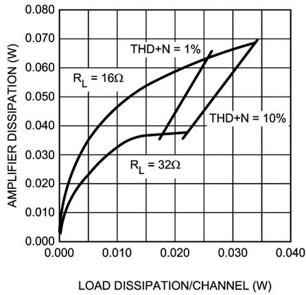
Amplifier Dissipation vs Load Dissipation
