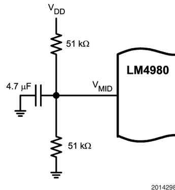
FIGURE 4. Simple circuit generates LM4980's  $V_{MID}$  voltage
