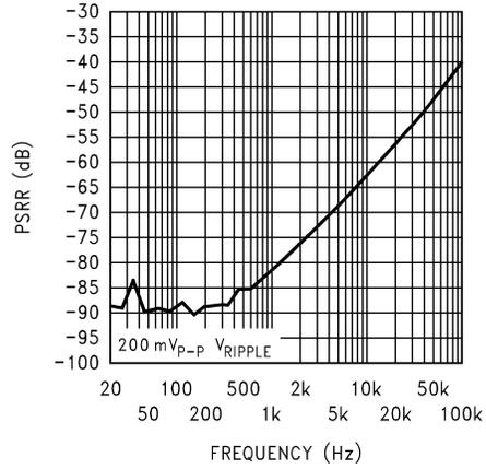
**Power Supply Rejection Ratio (PSRR)  $V_{DD} = 3V$
