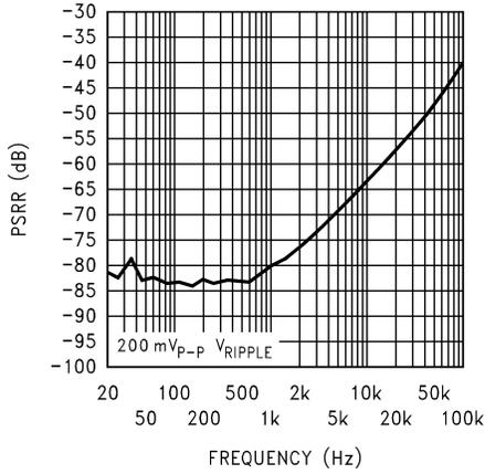
**Power Supply Rejection Ratio (PSRR)  $V_{DD} = 5V$
