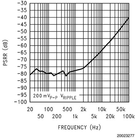
**Power Supply Rejection Ratio (PSRR)  $V_{DD} = 3V$
