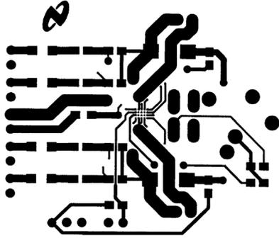
Figure 13. Recommended 20-pin micro SMD PC Board Layout:
