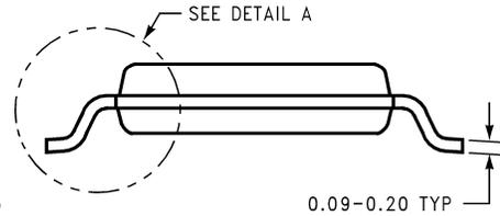
**20-Lead MOLDED TSSOP, EXPOSED PAD, 6.5x4.4x0.9mm**
