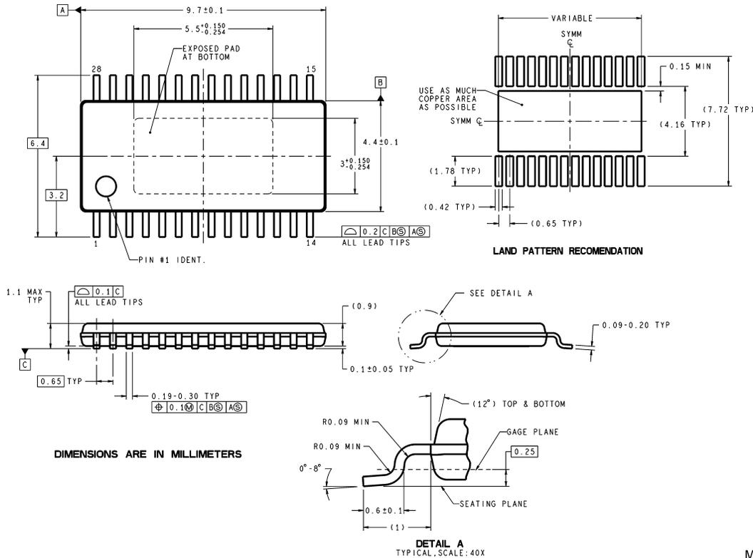
**28-Lead MOLDED TSSOP, EXPOSED PAD, 9.7x4.4x0.9mm**
