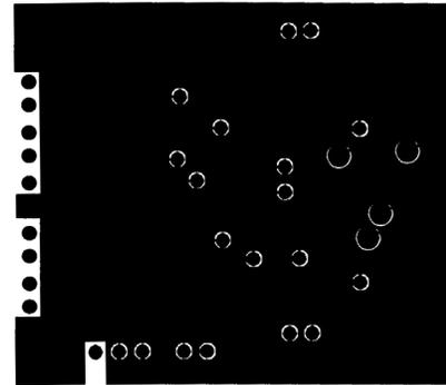
Figure 16. Recommended 20-pin micro SMD PC Board Layout:
