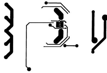
Figure 14. Recommended 20-pin micro SMD PC Board Layout:
