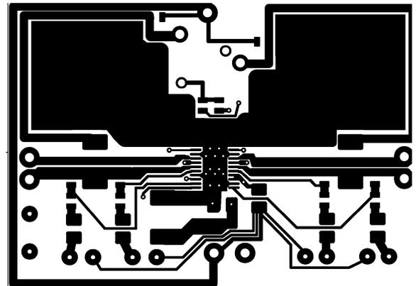
FIGURE 5. Recommended MTE PC Board Layout: Component-Side Layout
