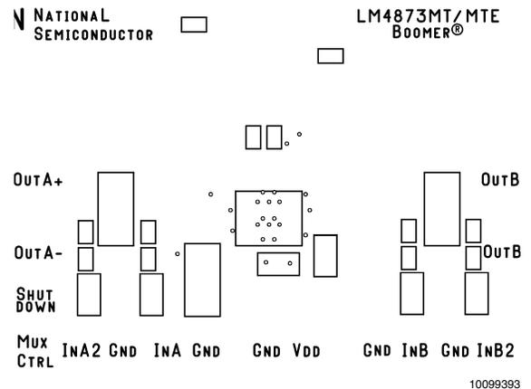
FIGURE 4. Recommended MTE PC Board Layout: Component-Side Silkscreen
