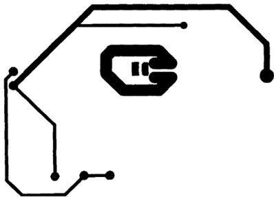
Figure 15. Recommended 20-pin micro SMD PC Board Layout:
