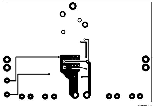
FIGURE 6. Recommended MTE PC Board Layout: Bottom-Side Layout
