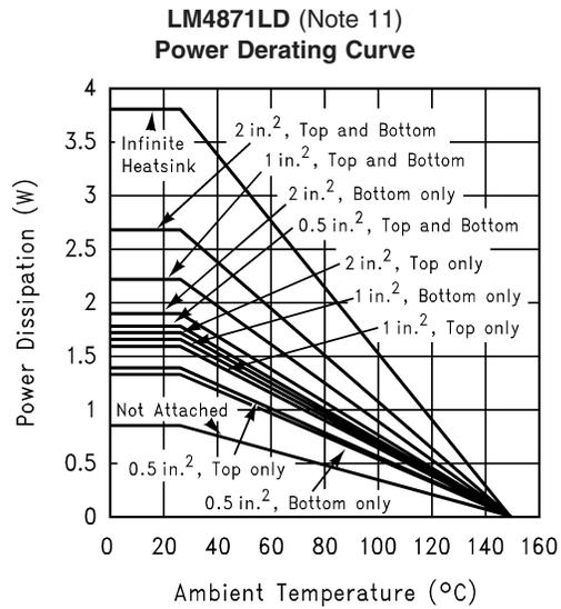
**Note 11:** This curve shows the LM4871LD's thermal dissipation ability at different ambient temperatures given the exposed-DAP of the part is soldered to a plane of 1oz. Cu with an area given in the label of each curve. This label also designates whether the plane exists on the same (top) layer as the chip, on the bottom layer, or on both layers. Infinite heatsink and unattached (no heatsink) conditions are also shown.
