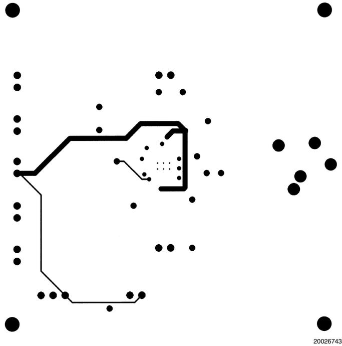
**FIGURE 12. Recommended LQ PC Board Layout:
