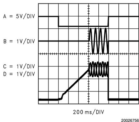
**FIGURE 2. Differential output signal (Trace B) is devoid of transients. The SHUTDOWN pin is driven by a shutdown signal (Trace A). The inverting output (Trace C) and the non-inverting output (Trace D) are applied across an  $8\Omega$  BTL load.**
