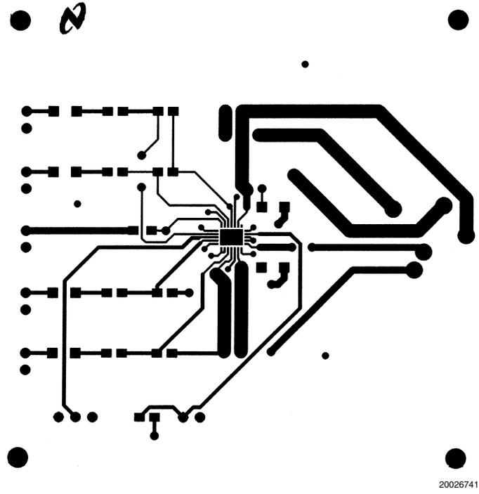
FIGURE 10. Recommended LQ PC Board Layout:
