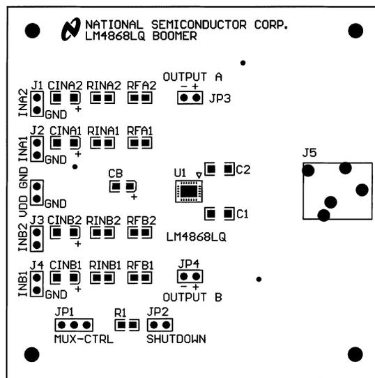
**FIGURE 9. Recommended LQ PC Board Layout:
