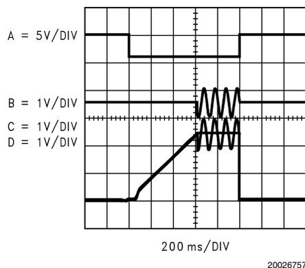
**FIGURE 3. Single-ended output signal (Trace B) is devoid of transients. The SHUTDOWN pin is driven by a shutdown signal (Trace A). The inverting output (Trace C) and the  $V_{\text{BYPASS}}$  output (Trace D) are applied across a  $32\Omega$  BTL load.**
