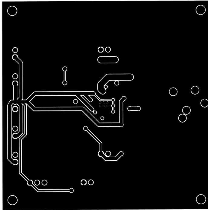
FIGURE 11. Recommended LQ PC Board Layout:
