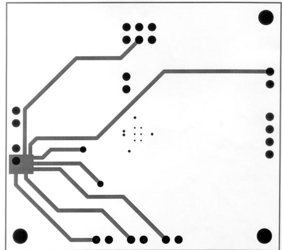
FIGURE 10. Recommended LD PC Board Layout: Inner Layer 2
