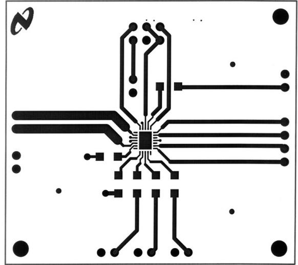
FIGURE 8. Recommended LD PC Board Layout: Top Layer
