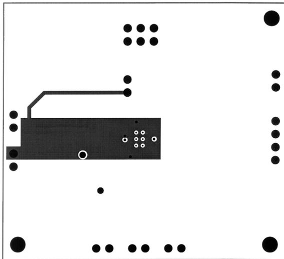
FIGURE 9. Recommended LD PC Board Layout: Inner Layer 1
