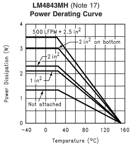
**Note 17:** These curves show the thermal dissipation ability of the LM4843MH at different ambient temperatures given these conditions:
