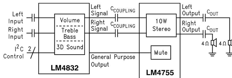
10W/ch System with I<sup>2</sup>C Controlled Tone, Volume and 3D Sound
