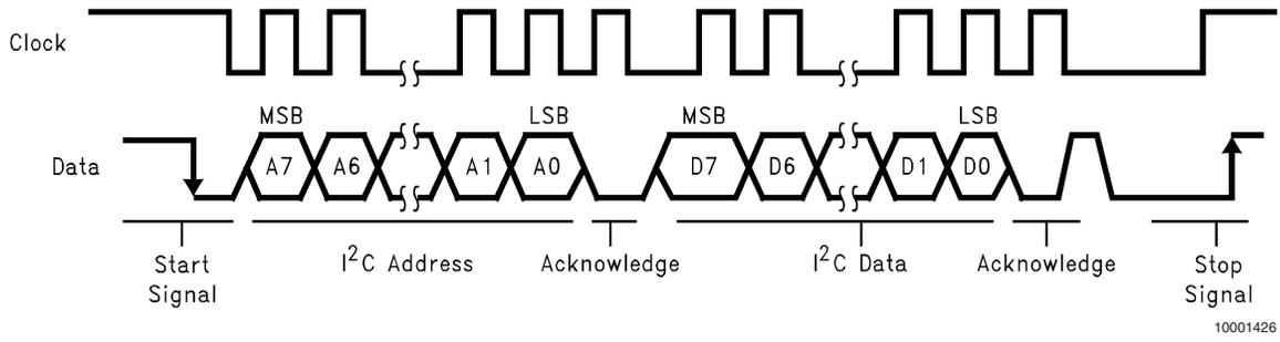
FIGURE 3. I<sup>2</sup>C Bus Format
