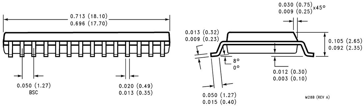
**28-Lead SOIC Package (M28B)**
