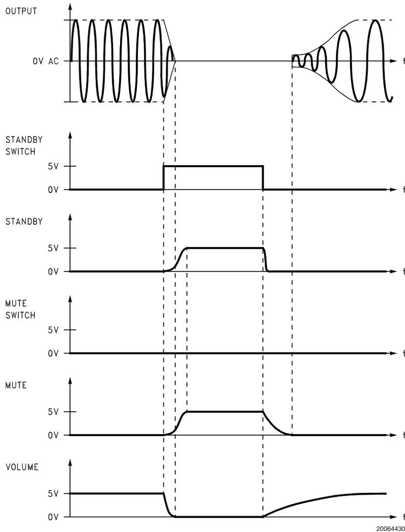
FIGURE 6. Turn-On/Off External Circuitry Sequence
