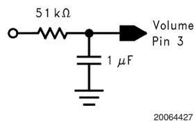
FIGURE 3. Volume Pin Lowpass Filter
