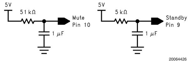
**FIGURE 2. Mute and Standby Pin Lowpass Filters**
