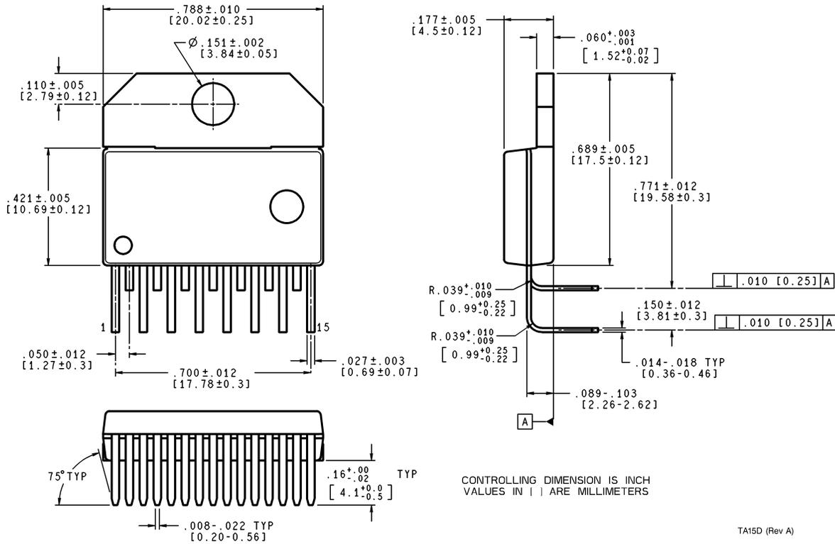
**Staggered 15 Lead Non-Isolated TO-220 Package
