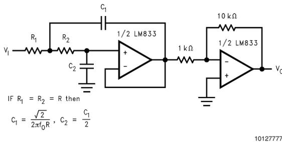
FIGURE 6. Pre-amplifier Stage with Low Pass Filter
