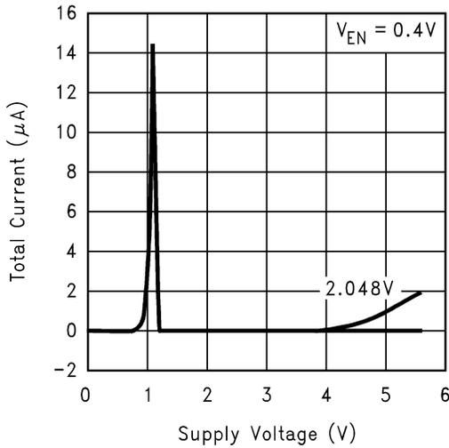
**Total Current ( $I_{S(ON)}$ ) vs Supply Voltage**
