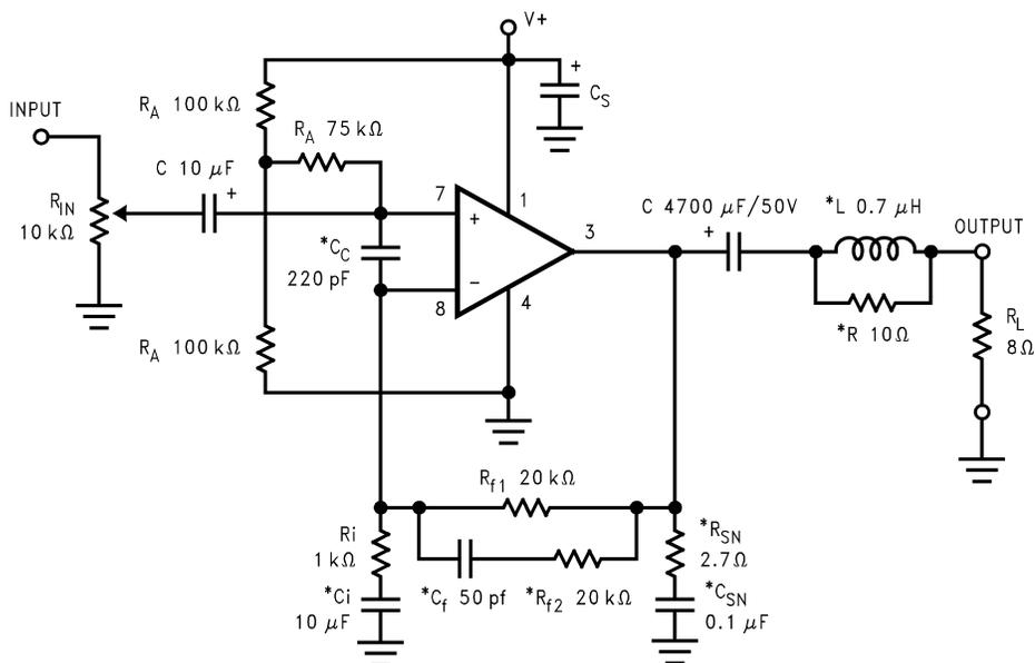
\*Optional components dependent upon specific design requirements. Refer to the External Components Description section for a component function description.
