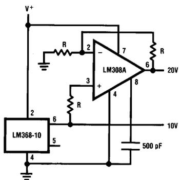
R = Thin Film Resistor Network
