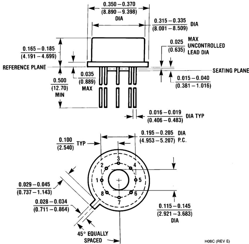
Thermal resistance is 45°C/W, junction to case, and 150°C/W, junction to still air.
