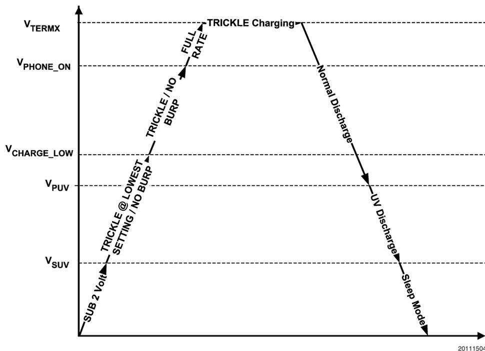
FIGURE 1. Voltage Thresholds
