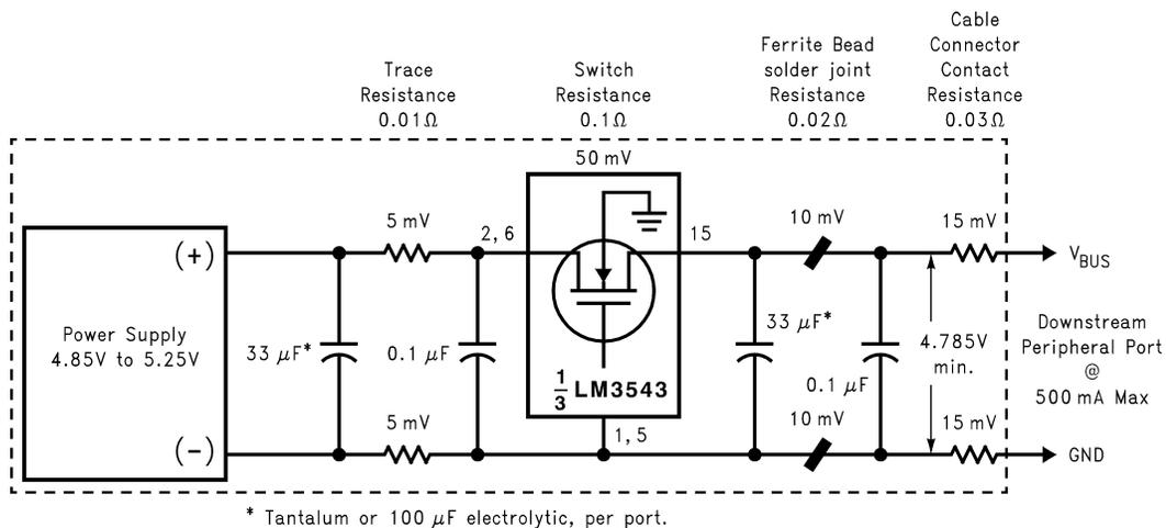
**FIGURE 6. Self-Powered Hub Connections and Per-Port Voltage Drop**
