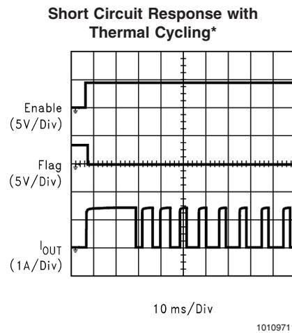
\* Output is shorted to Ground through a 100 mΩ resistor
