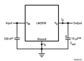
\* Required if regulator is located more than 2" from power supply filter capacitor.
