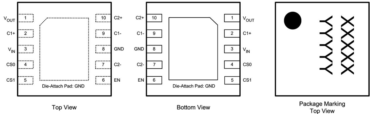
**Note:** The actual physical placement of the package marking will vary from part to part. The package marking placeholder "XXXXX" is a code for die traceability. "YYYYY" identifies the device (part number, voltage option, etc.). See the Order Information table below for the device ID codes.
