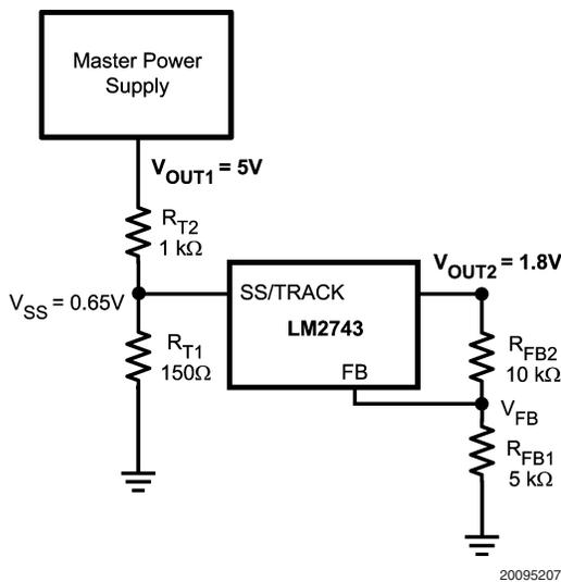
FIGURE 1. Tracking Circuit
