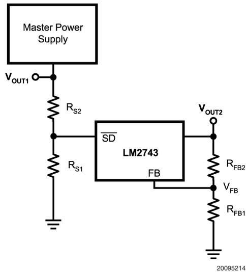
FIGURE 4. Sequencing Circuit
