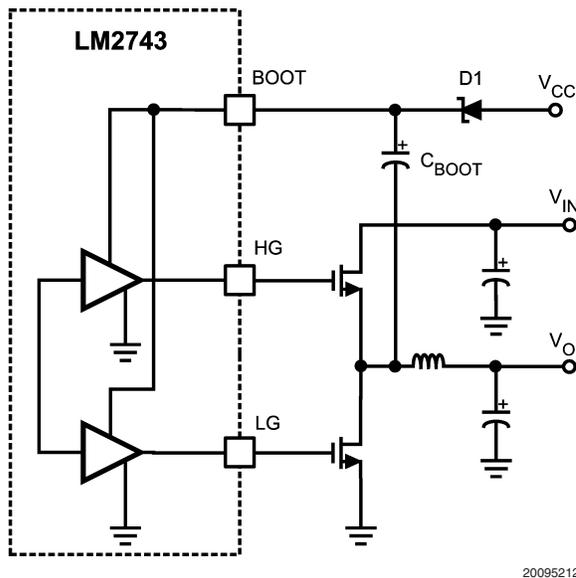
FIGURE 7. Basic Charge Pump (Bootstrap)
