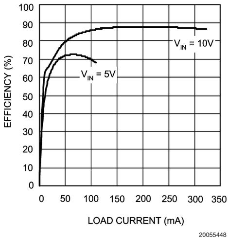
Efficiency vs Load Current ( $V_{OUT} = 35V$ ) - "X"
