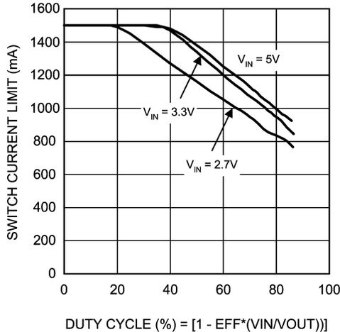
Switch Current Limit vs Duty Cycle - "X"
