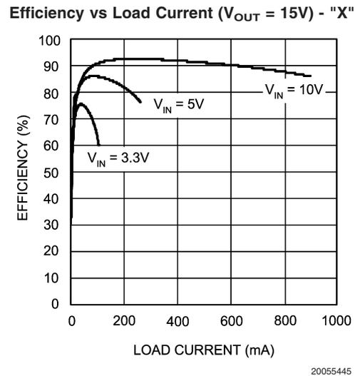
**Typical Performance Characteristics** Unless otherwise specified:  $V_{IN} = 5V$ , SHDN pin is tied to  $V_{IN}$ . (Continued)
