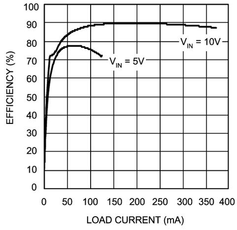
Efficiency vs Load Current ( $V_{OUT} = 30V$ ) - "X"
