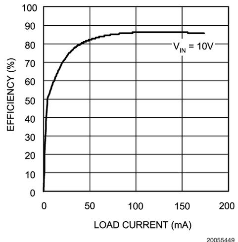
Efficiency vs Load Current ( $V_{OUT} = 40V$ ) - "X"
