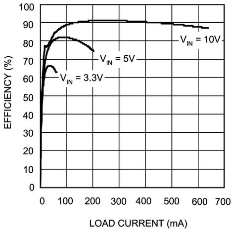
Efficiency vs Load Current ( $V_{OUT} = 25V$ ) - "X"
