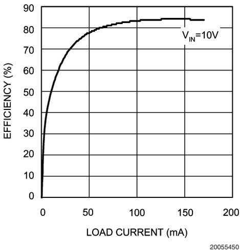
Efficiency vs Load ( $V_{OUT} = 15V$ ) - "Y"
