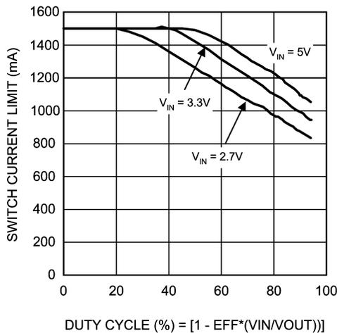
Switch Current Limit vs Duty Cycle - "Y"
