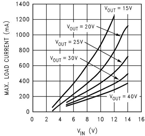
Max. Load Current vs VIN - "X"
