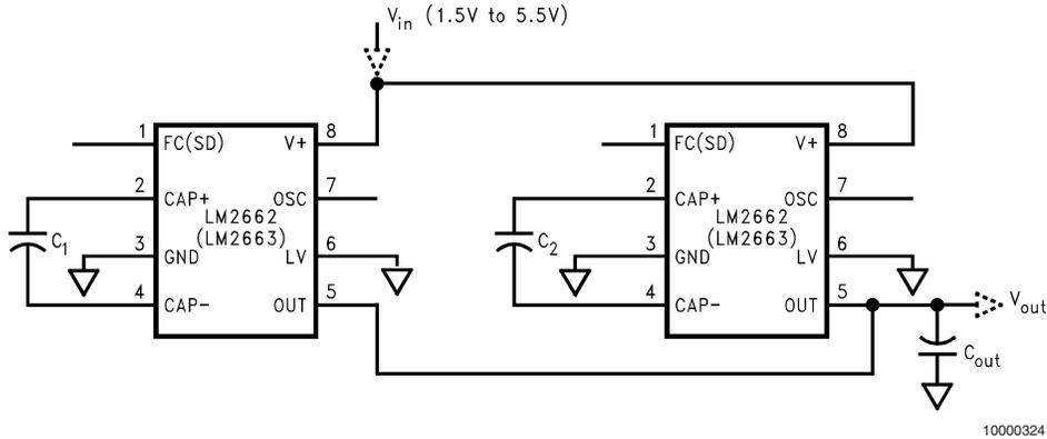
FIGURE 4. Lowering Output Resistance by Paralleling Devices
