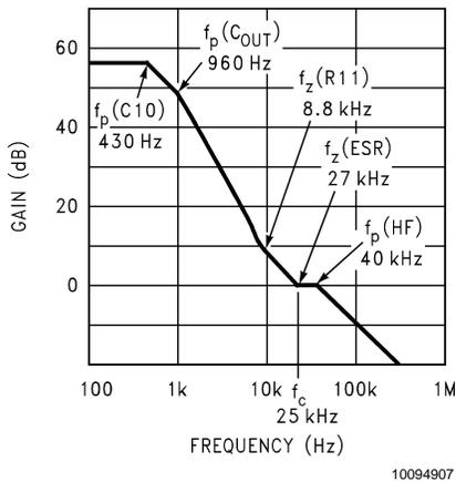
**FIGURE 6. Calculated Gain Plot for 3.3V/4A Application**
