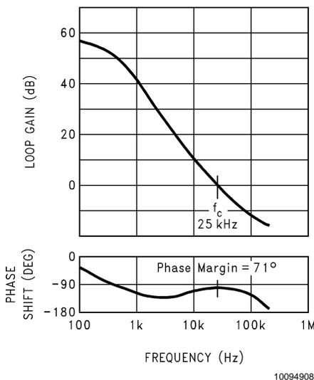
**FIGURE 7. Measured Gain/Phase Plot for 3.3V/4A Application**
