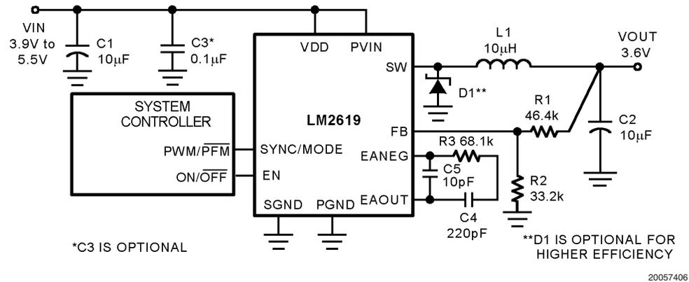
FIGURE 4. Typical Operating Circuit for 3.6V Output Voltage
