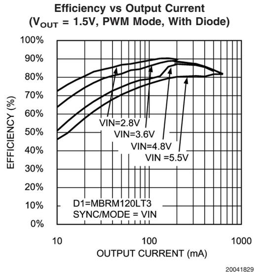
**Typical Operating Characteristics** LM2612ABL/ATL, Circuit of *Figure 1*,  $V_{IN} = 3.6V$ ,  $T_A = 25^\circ C$ ,  $L_1 = 10 \mu H$ , unless otherwise noted. (Continued)
