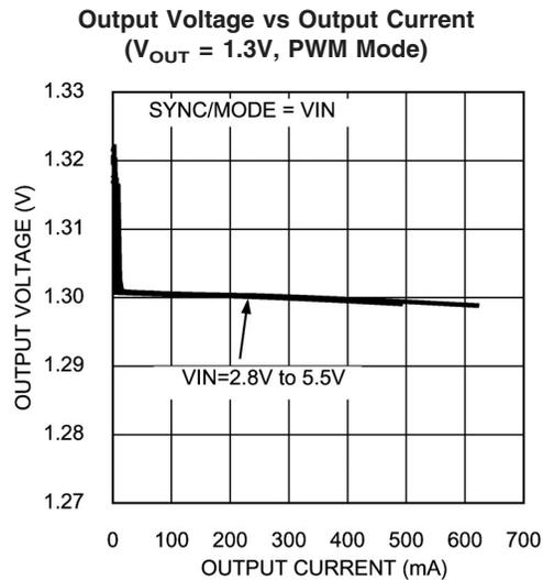
**Typical Operating Characteristics** LM2612ABP, Circuit of Figure 1,  $V_{IN} = 3.6V$ ,  $T_A = 25^\circ C$ ,  $L_1 = 10 \mu H$ , unless otherwise noted. (Continued)
