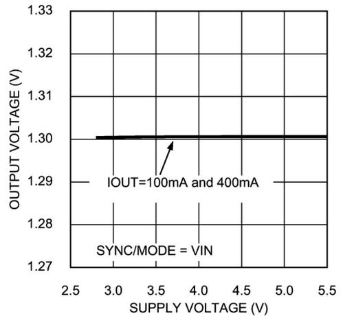
**Output Voltage vs Supply Voltage**
