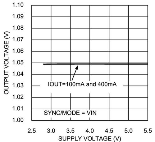
**Typical Operating Characteristics** LM2612ABP, Circuit of *Figure 1*,  $V_{IN} = 3.6V$ ,  $T_A = 25^\circ C$ ,  $L_1 = 10 \mu H$ , unless otherwise noted. (Continued)
