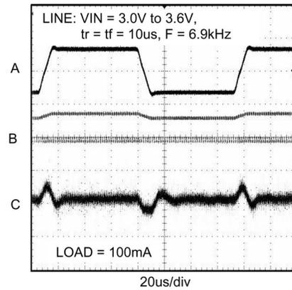
A: SUPPLY VOLTAGE, 500mV/div, AC COUPLED
