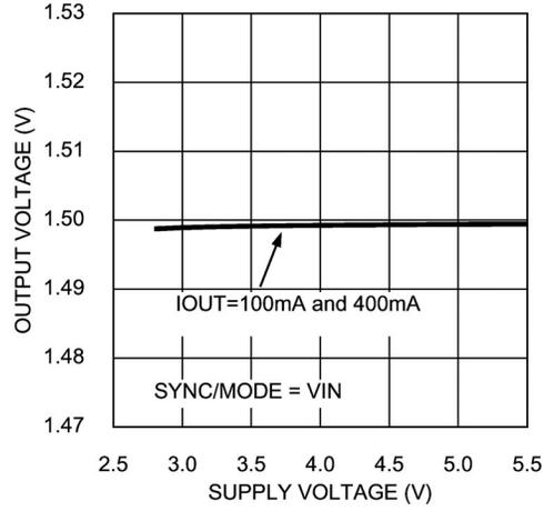
**Output Voltage vs Supply Voltage**
