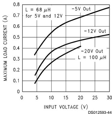
**FIGURE 28. Maximum Load Current for Inverting Regulator Circuit**
