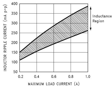
FIGURE 18. Peak-to-Peak Inductor Ripple Current vs Load Current
