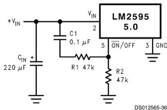
FIGURE 21. Delayed Startup
