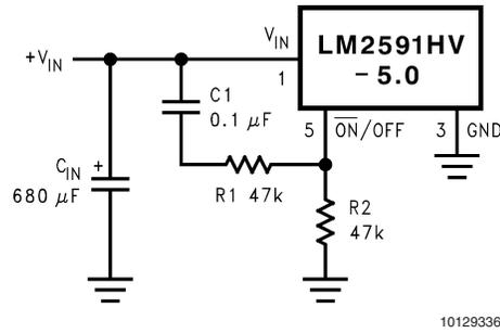
**FIGURE 7. Delayed Startup**
