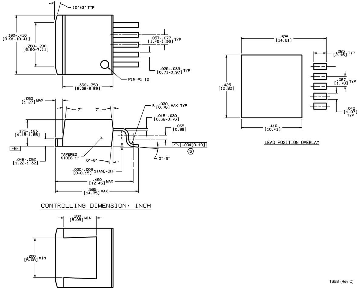
**5-Lead TO-263 Bent and Formed Package**
