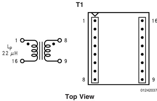
**FIGURE 21. Pulse PE-68411 (Surface Mount)**
