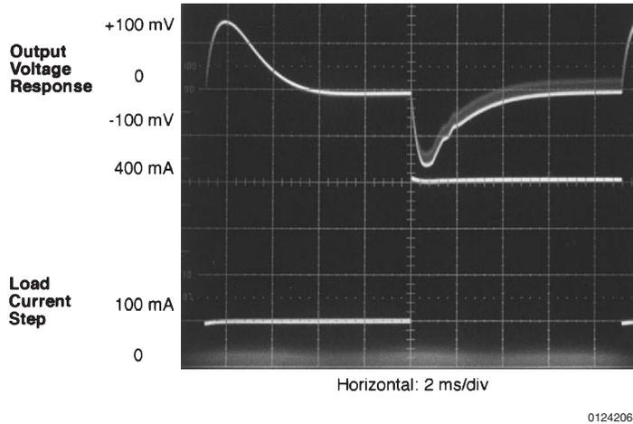
FIGURE 6.  $V_{OUT}$  Response to Load Current Step
