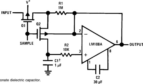
†Teflon, polyethylene or polycarbonate dielectric capacitor.
