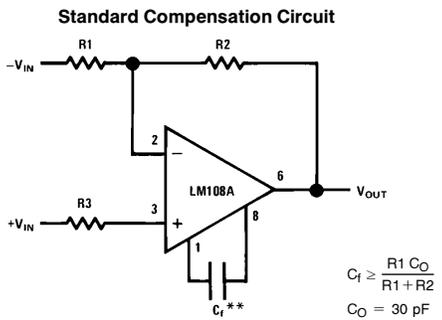
\*\*Bandwidth and slew rate are proportional to  $1/C_1$ .
