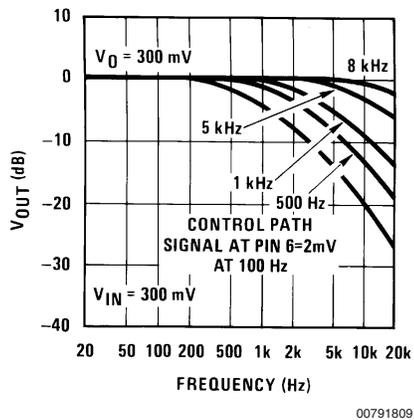
FIGURE 4. -3 dB Bandwidth vs Frequency and Control Signal
