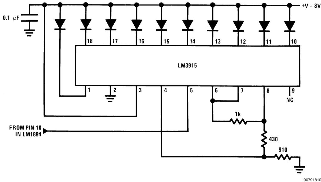
FIGURE 5. Bar Graph Display of Peak Detector Voltage
